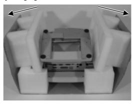
Take out the accessories/options from the partitions in the packaging materials and unfold the packaging materials carefully to unload the upsidedown loaded TP6000 series touch terminal. Put this main unit & paddle assembly aside for the whole Touch POS system installation. Collect if exist other options from the hidden compartments in the packaging materials like external FDD.
